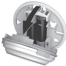
5. **Remove the protective tab between the batteries.**
