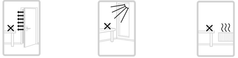
The T6 thermostat should not be placed near draughts, in direct sunlight or near heat sources.
