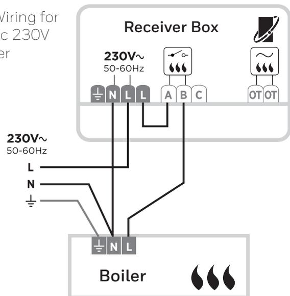
B) Wiring for Combi boiler
