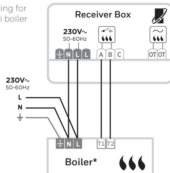
C) Wiring for OpenTherm boiler
