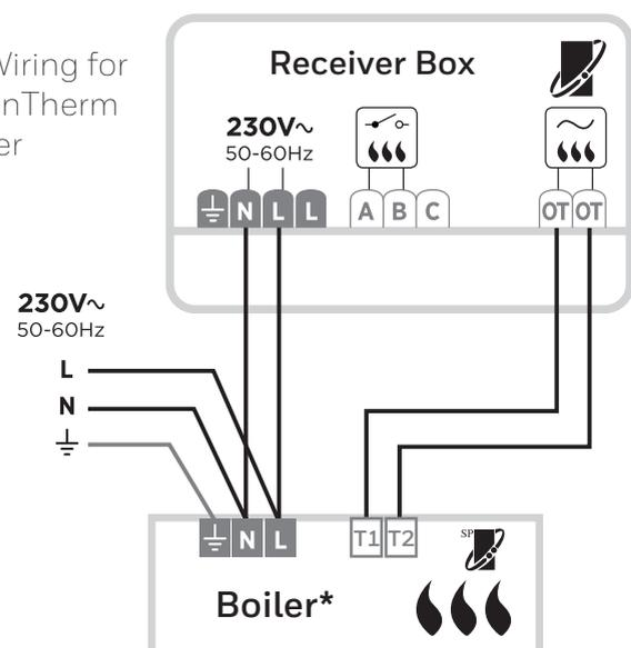
D) Wiring for two-port zone valve or S-plan
