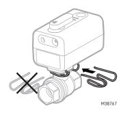
Fig. 4. Connect ball valve to actuator.
