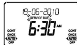
If the **SWITCH OFF** or **PROMPT** Actions have been selected, the „SERVICE DUE“ message will flash and the word "OFF" will appear on the display. The boiler has been switched off to ensure the safety of the User. A service appointment should be arranged immediately.
