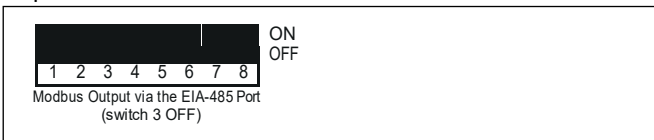
Fig. 14: DIP Switch Settings for Modbus Communications
