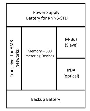
The transmitter and receiver are used to record and transmit data from the HCAs and then to forward this data to other nodes in the same network.
