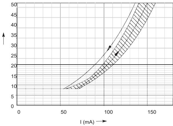
Pressure range 8 ... 50 mbar; Modureg upwards;
