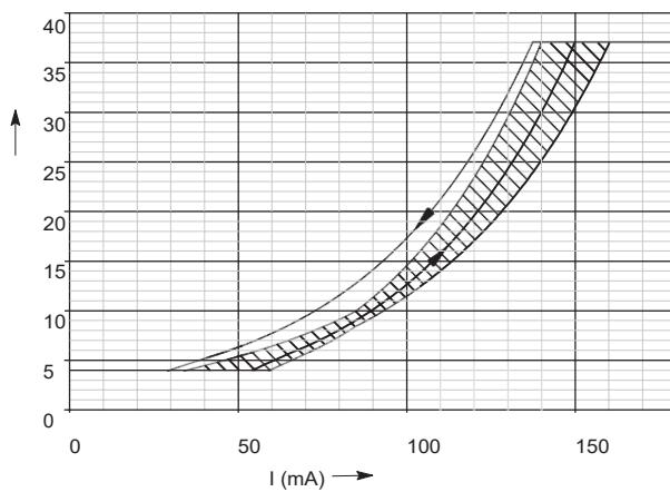
Pressure range 3 ... 37 mbar; Modureg upwards;
