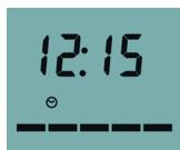
Pressing the [SET] key once enters the minutes and moves the display into the Set Hardness mode. This can be displayed in PPM, degrees German, or degrees French depending on the model of softener.
