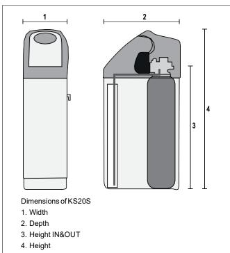
The softening device is controlled by a highly modern microprocessor. Using the integrated consumption counter the microprocessor calculates the individual consumption characteristics and the remaining capacities resulting thereof as well as the optimal time for the regeneration.
