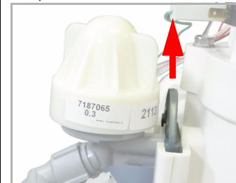
3. Pull off the ejector and the O-rings (Fig.1, pos. 1) and replace.
