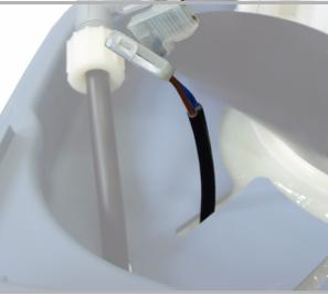
6. Release the hoses on the disinfection unit by pressing in the draw-off protection and gently pressing the hose in the direction of the disinfection unit. Pull off the hoses on both the infeed and the outfeed sides.
