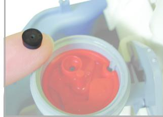
10. Insert the nozzle holding element.
