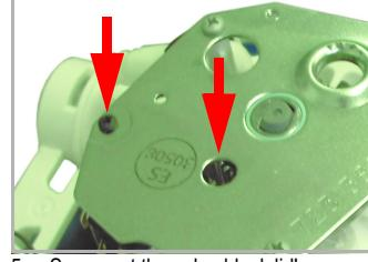
5. Screw out the valve block lid's screws and remove the lid completely.
