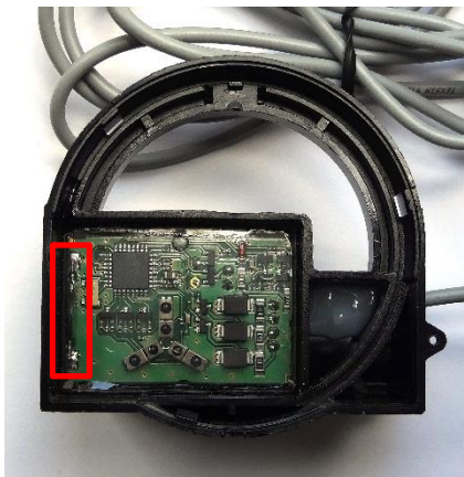
Figure 4. Position of reed switch in module EWA171C-PO
