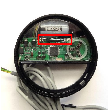
Figure 3. Position of reed switch in module EWA110C1520-PO and EWA110C2540-PO
