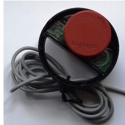
Figure 5. Briefly place magnet near reed switch
