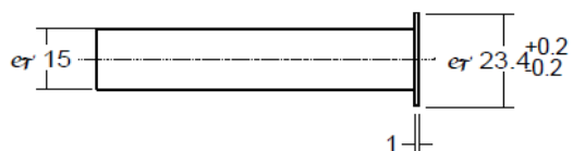
Fig. 10. Pipe (dia 18 mm) for flat sealing ring connection for G 3/4 " external thread
