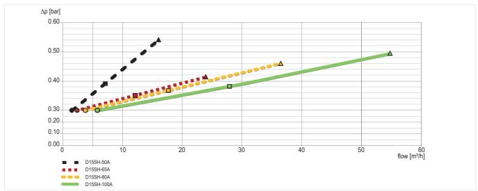
Fig. 2 Pressure drop within the valve in dependency of the flow rate and the used connection size (Sizes 50). Pressure setting: P1: 8 bar, P2: 3 bar
