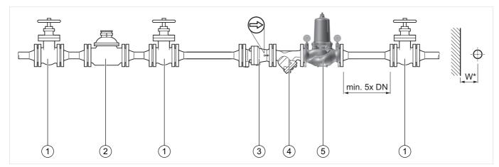
$\label{eq:Fig.1} \textit{Standard installation example for the pressure reducing valve}$
