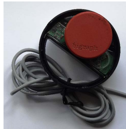
Figure 5. Briefly place magnet near reed switch
