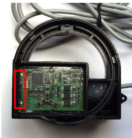
Figure 4. Position of reed switch in module EWA171C-MBUS
