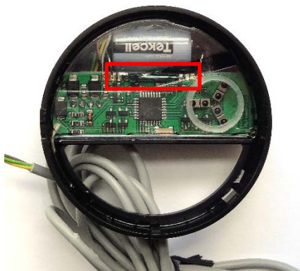
Figure 3. Position of reed switch in module EWA110C1520-MBUS and EWA110C2540-MBUS
