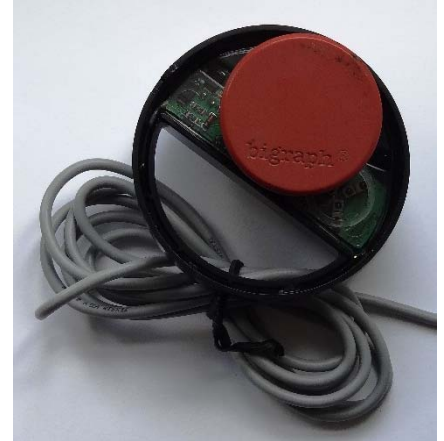
Figure 5. Briefly place magnet near reed switch
