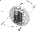
6. Attach the thermostat to the mounting plate.
